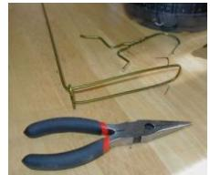
**Step 2:** Form a rectangle by making 90° bends. It should end up being about 1.5" wide by 6" long. Hint: make the first bend about 1" longer in order to form a clasp with the additional wire.
